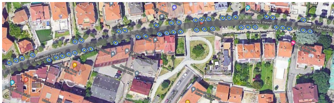
Figure 3: Parking sensors deployment in the Santander's downtown
